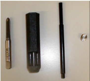
Repair Kit Contents 1 - M6X1 STI Tap 1 - Plastic tool (Not Used) 1 - Installation Tool 12 - Threaded Inserts
