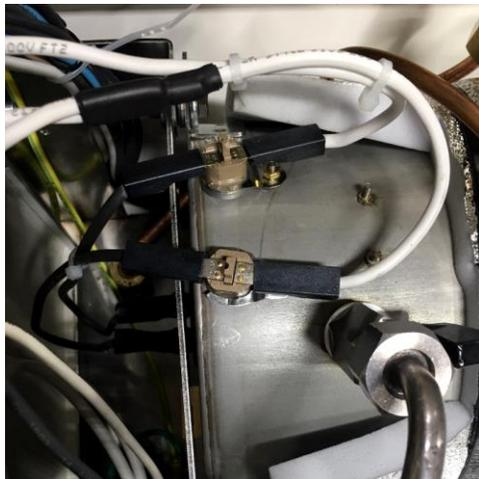
Additionally all two group Strada, Linea PB and Leva machines will now be equipped with two L276.01, Klixon trip free 130° thermostat.
