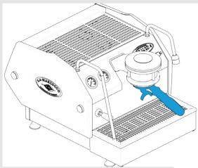
When the espresso machine is ready, place ground coffee into the portafilter and activate the brewing process. For additional information to operate this espresso machine please refer the the Owner's Manual or the Software Programming Guide.
