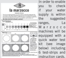
vou to check if vour water supply is within the suggested Ιa ranges, Marzocco machines will be equipped with a quick water test kit (see image below) including 6 test-strips and instruction cards. The parameters
