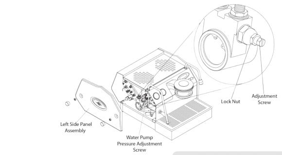
Figure 7 - Water Pump Pressure Adjustment
