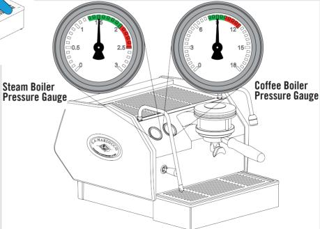
When brewing, the coffee boiler pressure should be between 8-10 bar. The steam boiler pressure should be set at 2 bar but can operate at any setting between 1.3 bar and 2 bar.
