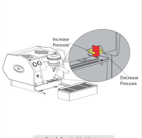
Figure 6 - Expansion Valve Adjustment
