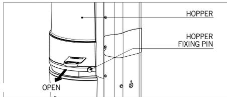
Make sure the hopper is positioned correctly on the appliance and fixed to the casing with relevant pins.
