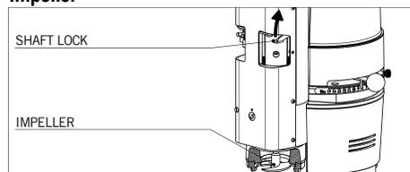
The impeller must be cleaned only by skilled technical personnel, **after disconnecting the appliance from the power supply**, according to the following instructions:
