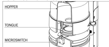
The system that protects against accidental contact with the rotating parts of the grinding system consists of a microswitch, situated under the body of the appliance, that cuts the electricity to the motor.
