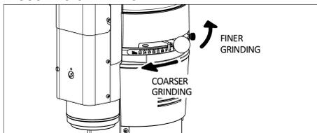
In order to achieve finer or coarser grinding, move the grinding adjustment level. To increase the coarseness of the ground coffee, the adjustment level must be rotated clockwise; to increase the fineness, turn the level anticlockwise.
