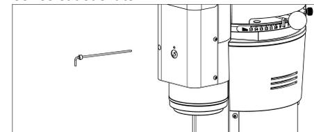
The cleaning of the coffee outlet chute must be made by the insertion of the tool 5.372.5 into the hole (caution when moving the tool).
