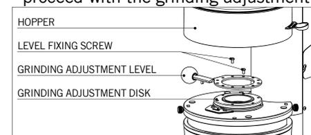
If the coffee comes out of the espresso coffee machine very quickly, it means the coffee is ground too coarse. Vice versa, if it comes out too slowly, it means the coffee is ground too fine. Nonetheless, bear in mind that there are many conditions liable to influence the correct supply, such as the weight of the portions, the compacting, the espresso machine settings, and the cleaning of the filters.
