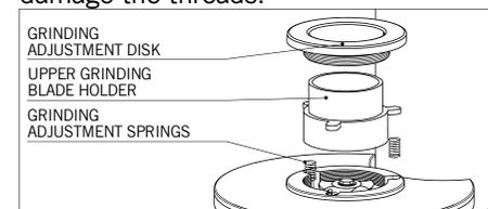
Please check that the grinding adjustment springs are on their place. Having refitted the upper grinding blade holder in the relevant slot, please lubricate, with grease suitable for food contact, the threads of the grinding adjustment disk and its underneath surface which touches the upper grinding blade holder. Screw the adjustment disk by turning it anticlockwise, place the adjustment level and fix it on adjustment disk with the relevant screws
