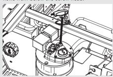
Tighten the screw to stop the water from flowing. Over tightening can cause damage to the sealing washer and the group cover. Repeat this procedure for all groups. Once all air is removed from the coffee boiler, reinstall the group cover by following the removal instructions in reverse.
