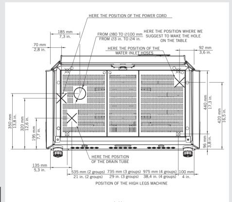
Fig. 2 - Installation guide
