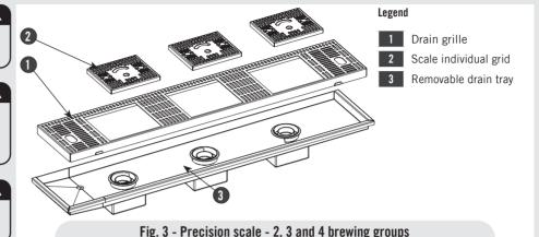
in the figure below, gently clean and dry them with an absorbent paper cloth. Dirt build-up or water stagnation may prevent the scale individual grid from properly settling into place.
