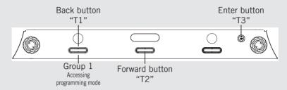
The keypad has two functions. The first is for control of the espresso. The second is for programming individual software parameters.
