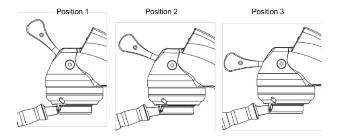
The Modbar espresso tap is able to command multiple functions using a single handle. We do this by combining the movement of three handle positions, as illustrated in the above diagram. Following are instructions for operating each of the tap functions.
