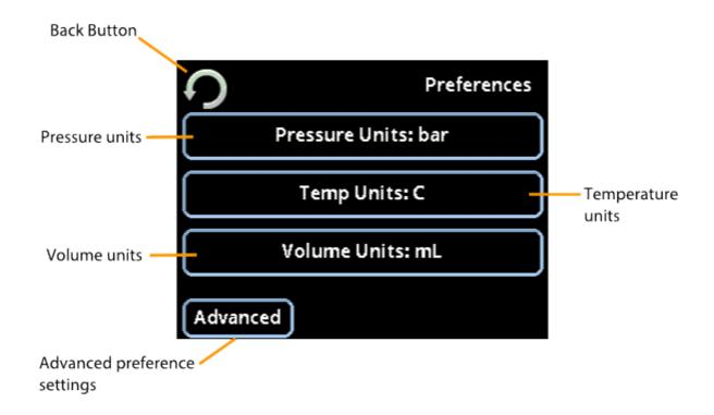
**Pressure units:** This button sets the system's pressure units, in: bars or psi
