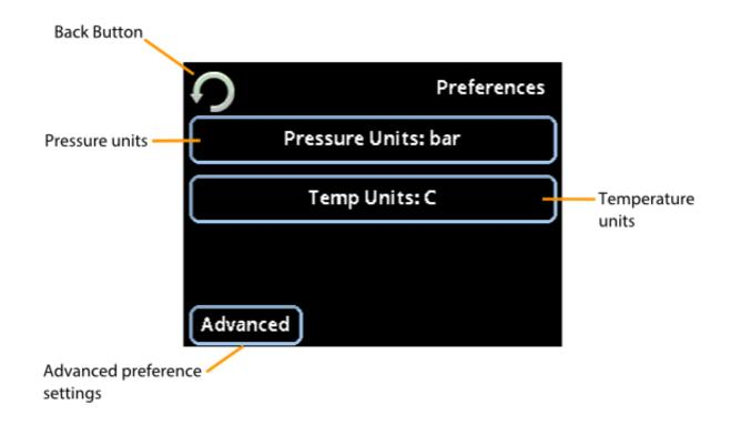
**<u>Pressure units:</u>** This button sets the system's pressure units, in: bars or psi
