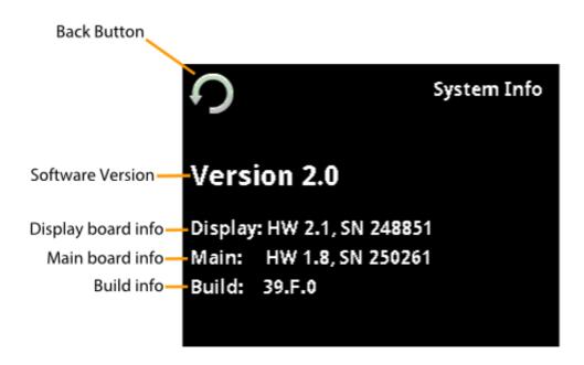
**Software Version:** This field displays the current software version loaded on the machine.
