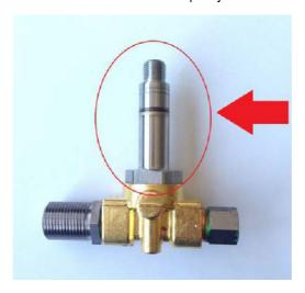
To help mitigate the issue, La Marzocco has improved the material of the two-way solenoid plunger sleeve from 303 series stainless steel to 316L series stainless steel. This improvement was introduced to machines manufactured in March 2015 starting with serial number Strada 1936, Linea PB 1767, GS3 5048, GB5 012944, Linea Classic 044938.
