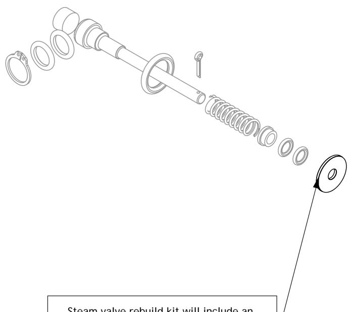
Steam valve rebuild kit will include an additional part with the following item code: L165/9B
