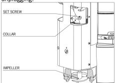
It is possible to change the dosage quantity by raising or lowering the height of the impeller.
