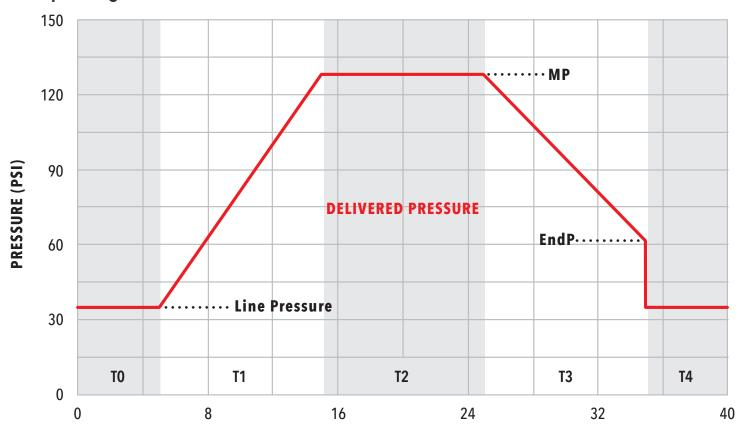
**TIME (SECONDS)** total time is variable and additive (total of T0 thru T4)
