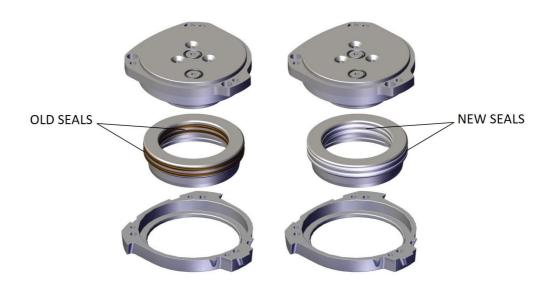
The new seals are available in the piston rebuild kit, code 1205, and in the piston assembly, which changes its part code from SA292 to SA292.01.
