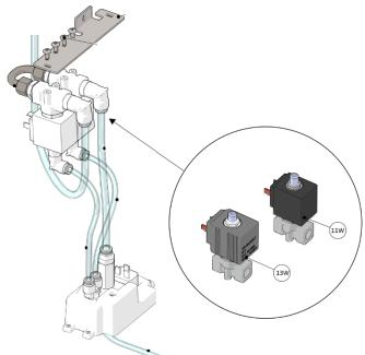
With the back cover removed, the inlet valve (11W) is on the right; and the purge valve (13W) is on the left.
