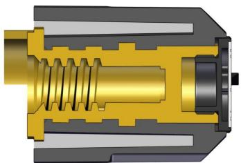
The new plastic cap is in contact with the metal plate only on a thin rim. The air gap limits heat transmission and drastically reduces the temperature of the plate.
