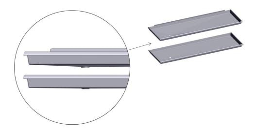
To retrofit the new tray in older machines, it may be necessary to slightly bend the brew valves drain tube backward, due to the presence of the higher wall.
